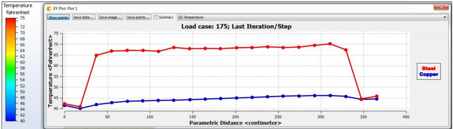
**Chill Roll Simulation - Copper vs. Steel:** In this CFD Model, all factors are the same (line-speed, heat load, flow-rate, etc.), except the roller shell material. The copper roll is running up to 30 degrees (F) cooler! Now the converter has the option of increasing his line-speed.
