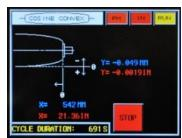
Menges' computer-controlled crown forming machines have the ability to create precision crowns as slight as .001 inch.
