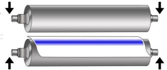
Menges Proof-Nip Impression Paper is easy to use. The nip system is simply opened, the paper slid between the rollers length-wise, and the nip system engaged. When the nip is opened, the paper shows very clear impressions indicating areas of high pressure and low pressure along the nip line.
