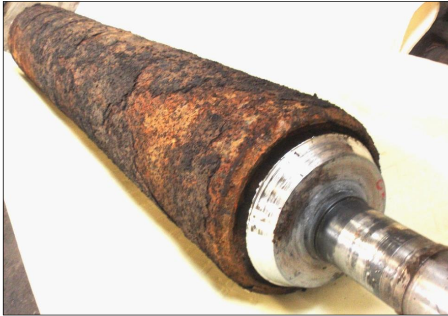
Figure 2. This shows the inner shell of a double-shelled chill roll that has been dissected as part of a rebuild. The roll functioned well for years, but the converter claims the roll doesn't perform like it used to: not a surprise.
