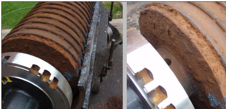
Figure 2. This double-shelled thermal roll played a critical role at its plant, so it was not regularly acid flushed, which would have been disruptive, requiring removal of the roller. As a result, rust and debris built up, and a complete inner shell rebuild was needed.
