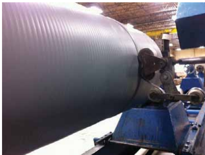
FIGURE 2. “Strip”-built rubber-roll covering
