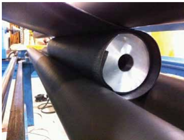
FIGURE 1. “Calender”-built rubber-roll covering
