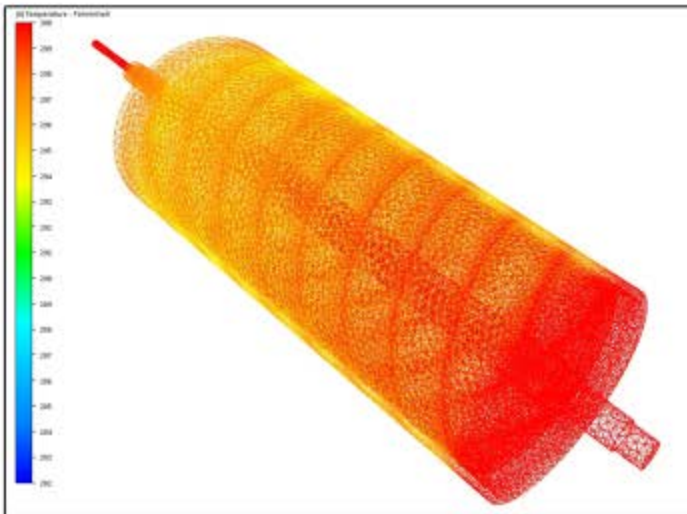
FIGURE 3. Hundreds of nodes along the rollface note exact temperatures externally and in the internally cavity of the roll.
