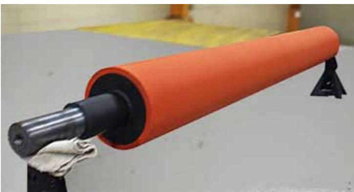
*Figure 6. Coating line roller with a newly-applied high-release silicone roll cover.*
